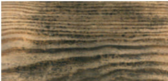
Untreated wood Showing Mold infestation after one year of external weathering in a moist climate
